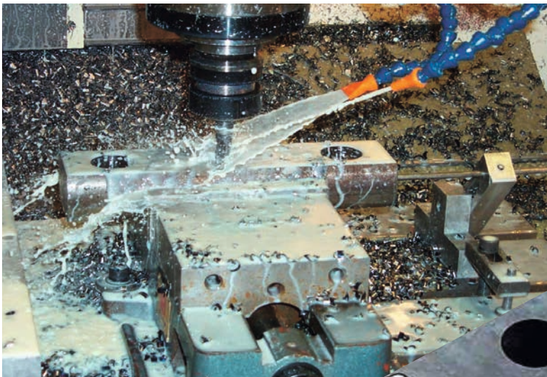
Manufacture of a Nobles 10 tonne Stainless Steel Tension Cell
