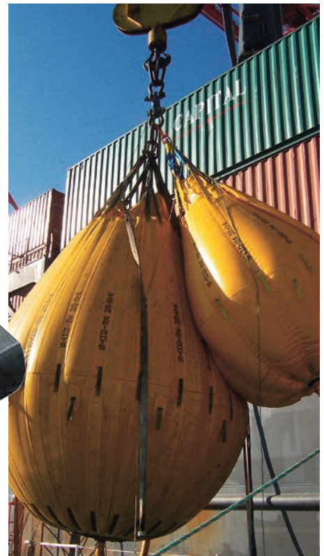
Nobles Tension Load Cell being used with Water Weights to proof load test a ship crane.
